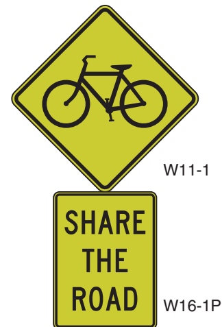
Figure 4-1. “Share the Road” Sign Assembly
